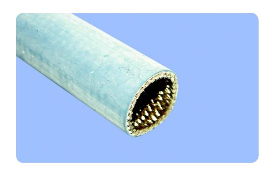
**Ben-Har™ 1151-FRB Grade B** is a rugged, flame-retardant, silicone rubber coated sleeving that provides excellent cut-through and abrasion protection for wiring systems in applications with temperatures ranging from -70°C to +200°C. Because the specially formulated silicone rubber is extrusion coated over the non-combustible fiberglass braid, it results in a reinforced sleeving that is superior to ordinary dip-coated sleeving and unreinforced rubber or plastic tubing.
