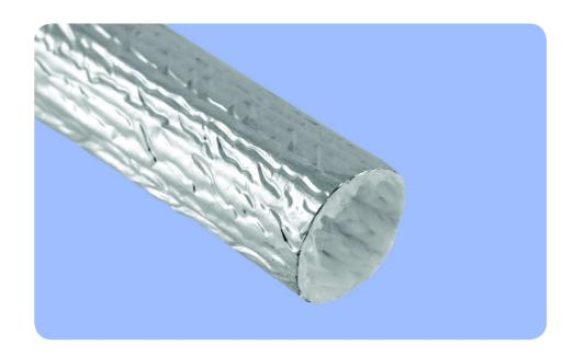
**ReflectSleeve® 1451** is a one-piece fiberglass sleeve that is laminated to an aluminum foil. A special manufacturing process permits the sleeve to boast a virtually seamless and non fraying construction. This feature makes ReflectSleeve 1451 a low profile solution easily applied to the application it protects. The outer aluminum finish is highly reflective while the inner layer of the fiberglass greatly increases insulating efficiency.
