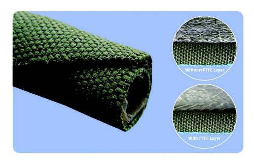
**ROUNDIT® 2000 NX EMI** is a self-wrapping sleeve designed for mechanical protection and EMI shielding of wire and cable bundles. The outer layer, which supplies the abrasion resistance, is manufactured from PPS monofilaments and Nomex® with an oil and water repellent treatment. The inner layer is composed of nickel-plated copper (Cu/Ni), which provides EMI insulation. The outer layer construction with a 100% covering ratio provides excellent cut-through and abrasion resistance.
