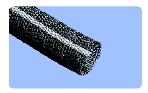
**ROUNDIT® 2000 V0** is a wrappable sleeving manufactured from flame retardant polyester monofilaments. ROUNDIT 2000 V0 is designed for mechanical protection and maintenance of wire and cable bundles and has an excellent cutthrough and abrasion resistance.
