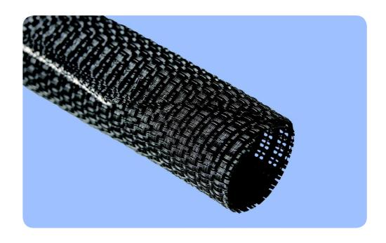
**ROUNDIT® PPS** is a self-wrapping sleeve manufactured from polyphenylene sulfide (PPS) monofilaments. This product offers excellent off-gasing properties and does not absorb or trap moisture making it ideal for use in space applications. The design allows for quick and easy installation and removal for the assembly, maintenance and inspection of wire harnesses and cable assemblies.
