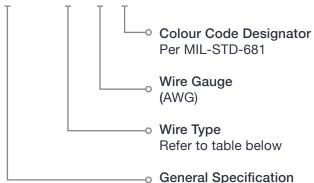
SAE AS81044 wire is an extremely versatile and reliable stranded single-conductor insulated lead wire with an impressive operating range of -65°C to 150°C and a maximum voltage rating of 600V. This wire offers a resistance to cut-through, abrasion, cold flow and common chemicals, and has low smoke characteristics. This wire is ideal for cable construction, routing in conduits, or in protected areas of avionics and airframe compartments.
